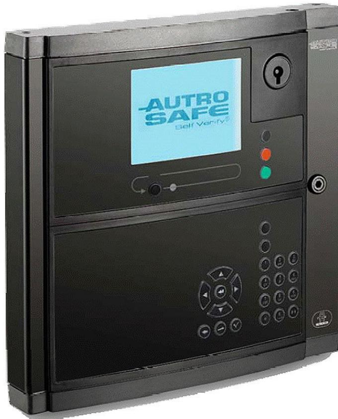
AutoSafe interactive fire-alarm system is a system where all system units communicate on a local network called AUTROLON. The system complies with C.E.N. EN 54 regulations. The SelfVerify function makes the system capable of every day to inspect and verify its own configurations, alarm and warning levels, interfaces and connection cables - from detector's sensing element to the alarm output.
