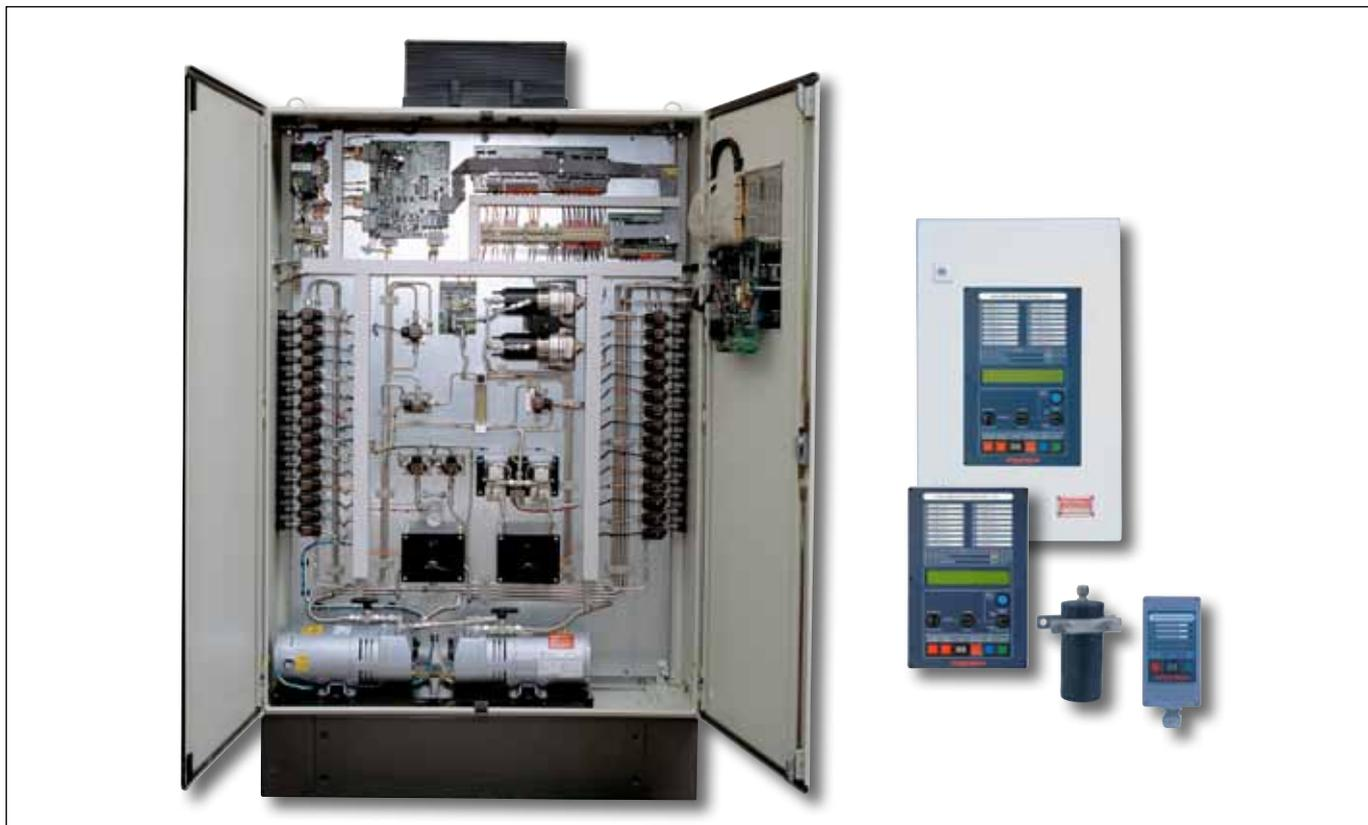
Gas Sampling System OGS 3.1 is our advanced model for special requirements. Different models and options cover most applications onboard any kind of tankers with special needs. All delivered parts are completely assembled ready for interconnection to on-site application. OGS 3.1 is based on a scanning method, which means that sample points are being connected to sensor(s) in a cyclic sequence. The operator panel has LCD display and individual LED lamps indicating each measuring point status.
